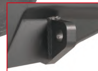
D-RING MOUNTS WELDED INSIDE AND OUT
