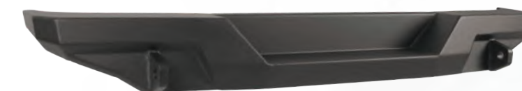
D-RING MOUNTS WELDED INSIDE AND OUT
