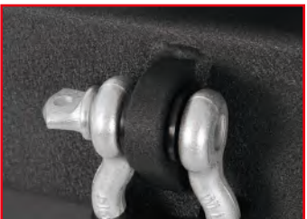
D-RING MOUNTS WELDED INSIDE AND OUT
