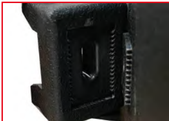
EXTERNAL REINFORCEMENT TO SUPPORT 40" TIRE
