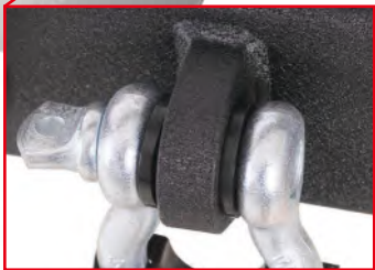
D-RING MOUNTS WELDED INSIDE AND OUT
