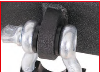
D-RING MOUNTS WELDED INSIDE AND OUT
