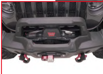
REMOVABLE OVERRIDER FOR LOW PROFILE DESIGN
