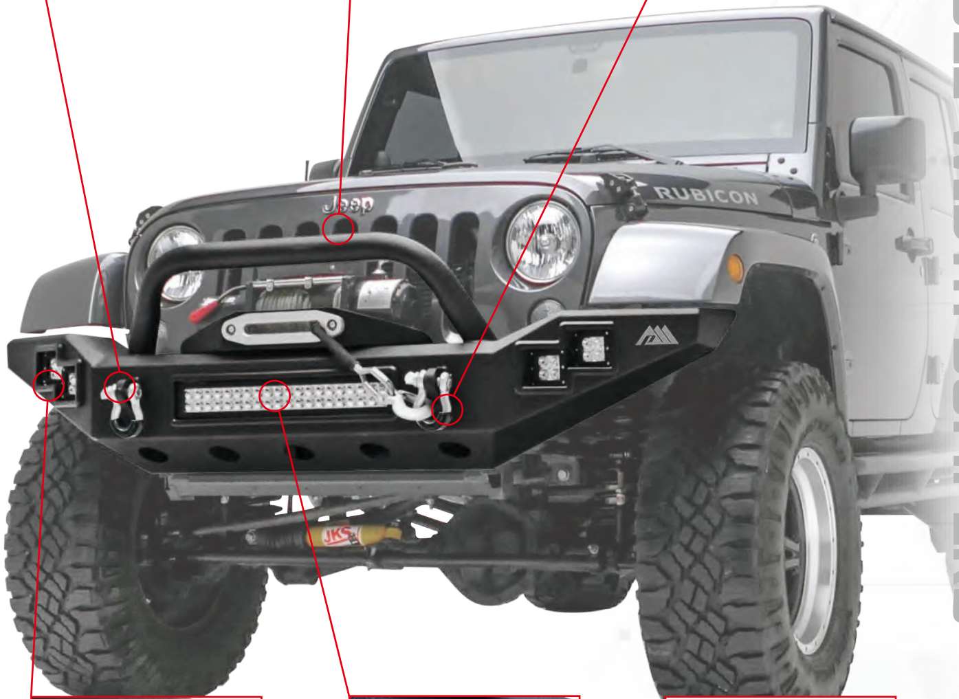
D-RING MOUNTS WELDED INSIDE AND OUT
