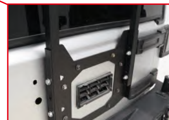
USES OE MOUNTING LOCATION NO DRILLING
