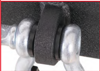
D-RINGS MOUNTS WELDED INSIDE AND OUT
