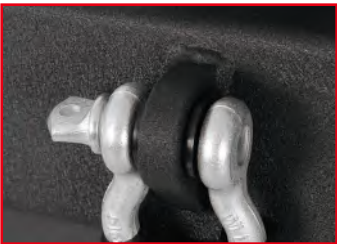
D-RING MOUNTS WELDED INSIDE AND OUT
