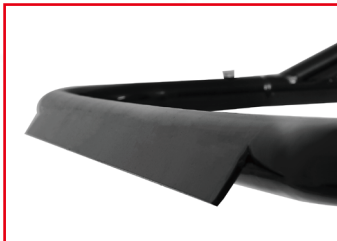
WIND DEFLECTOR ELIMINATES CAB NOISE
