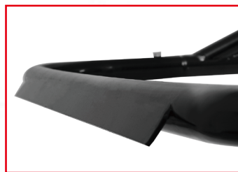
WIND DEFLECTOR ELIMINATES CAB NOISE
